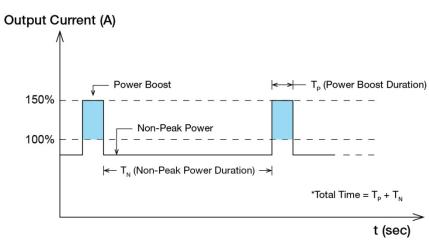
Fig. 3 Duty Cycle Calculation
