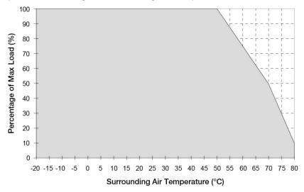
Fig. 1 De-rating for Vertical Mounting Orientation
