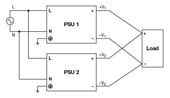
Fig. 5 Parallel Operation Connection Diagram
