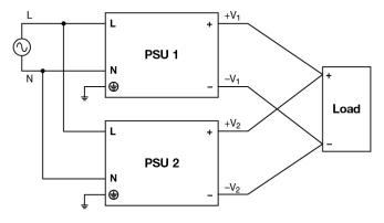
Fig. 5 Parallel Operation Connection Diagram
