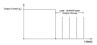
It is not recommended to prolong the duration of  $I_{\rm O}$  when it is less than OLP/OCP point, but greater than 100%, since it may cause damage to the PSU.
