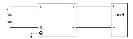
Fig. 6 DC Input Operation Connection Diagram
